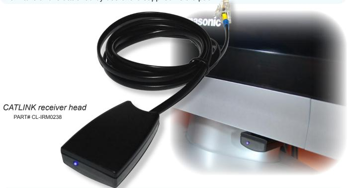
Equipped with a blue 'Talk-back' indicator light which flashes whenever infrared signals are received.
