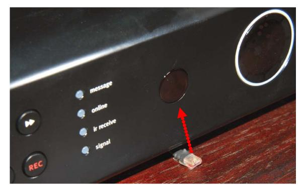
In this arrangement the domed face of the emitter is pointing up to the IR reception window.
