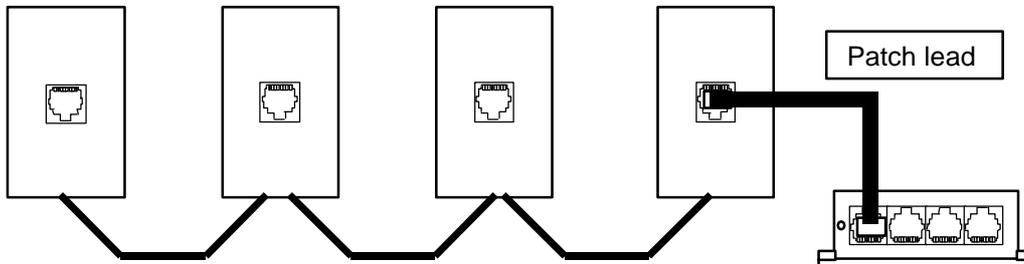
Connection of the Emitters and Receiver Heads is done by just plugging them into the desired wall plates – no other cabling required.
