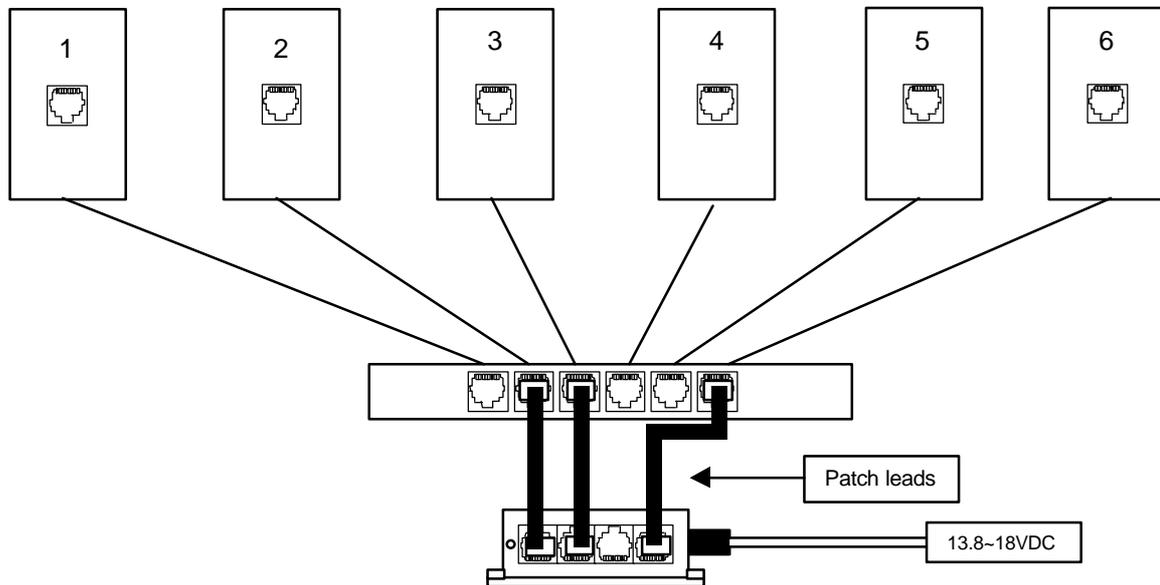
The number of outlets supported can be extended beyond the four provided by the distribution hub by providing option in the patch panel for parallel connection of outlets to a single Hub socket. Do not attach more than 6 outlets to a distribution hub port.
